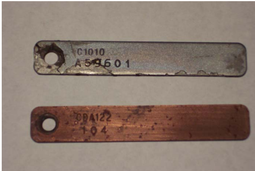
Photos 6: Coupons – 157 Days Exposure - After Cleaning
