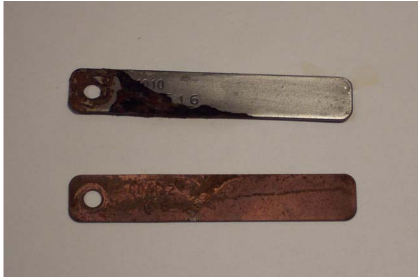
Photo 2: Coupons – 63 Days Exposure - Before Cleaning
